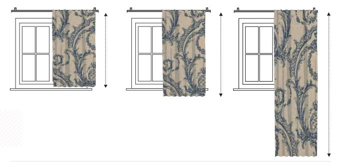
Sill Length 1cm above the sill Below sill length 15cm below the sill Full length 1.5cm from the floor
