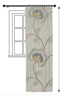
Sill Length 1cm above the sill Below sill length 15cm below the sill Full length 1.5cm from the floor
